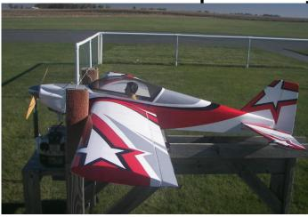
The plane is an Escapade 30cc made by Great Planes. It is powered by a DLE 35cc engine. The control surfaces are powered by Futaba S3305 servos (high torque, metal gear) and the choke and throttle Futaba S3010 servos. I fly my fueled aircraft with a Futaba 14SG transmitter and the Escapade uses an 8 channel receiver.
