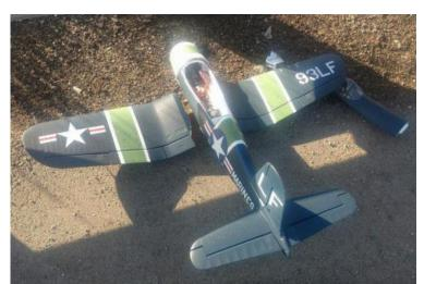
The picture on the road is how we found it, the left wing was separated but the two spars were not broken. The underside of the fuselage at the nose sustained damage, the wing bolt attachments are loose, I won't know how repairable that is until I remove the wing. The replacement fuselage and wing are \$72 each so if the repairs don't come out to my satisfaction I'll replace them with new parts.
