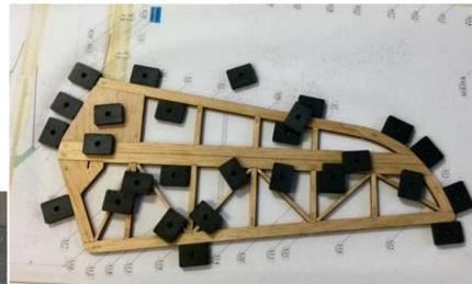
laser cut parts that fall out of the balsa sheets and the laser cut stringers. Everything you see in the pictures was precut, I didn't have to do anything to the parts.
