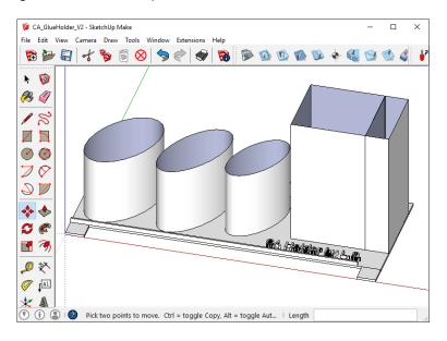
Now for the 3D print. 3D printing is painfully slow. It takes about 2 ½ hours to print the drawing above. The print run below is creating 2 glue holders. Each printed layer is .3 mm thick and .4 mm wide. Each unit takes **23 meters** of 1.75 mm PLA filament to build it. The units below are version 2. The drawing above is version 3 and has an extra slot for pencils, knives, etc.
