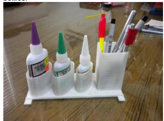
Total print time for 2 holders is about 5  $\frac{1}{2}$  hours. Here are the completed holders:
