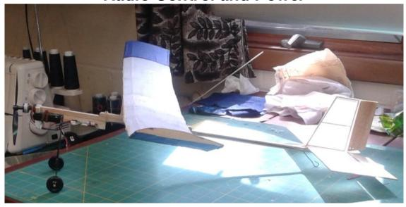
The model was originally a Sig Cub. It started with a 24 inch wing with dihedral but I added another 6 inches of wing and polyhedral. I also added area to the tail surfaces and gave it an elevator. The electronics came from an old UMX GB R2. Much to my surprise, it flies wonderfully, very stable and gentle like the rubber band powered model.
