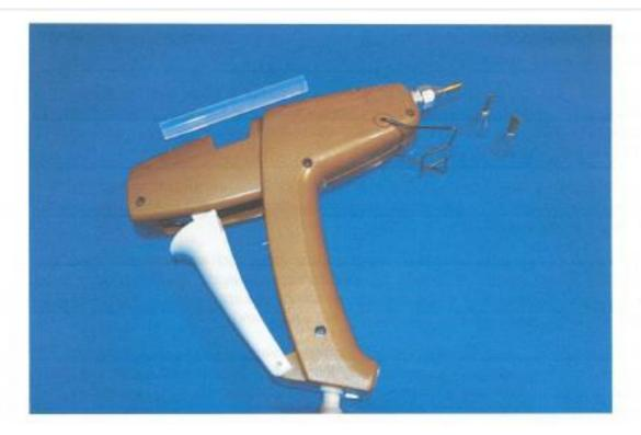
Hot glue is handy for quickly assembling sheet-foam models. This fancy glue gun has a variety of applicator tips. Even inexpensive glue guns are effective.
