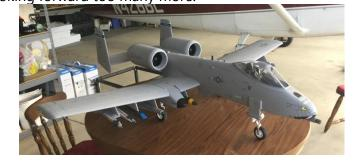
I'm running a pair of Admiral 6 cell, 5000mAh, 50C batteries. My timer is set at 3:30, when the timer
